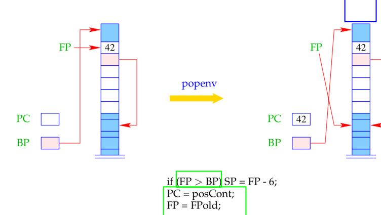
If popping the stack frame fails, new data are allocated on top of the stack. When returning to the frame, the locals still can be accessed through the `FP`!
