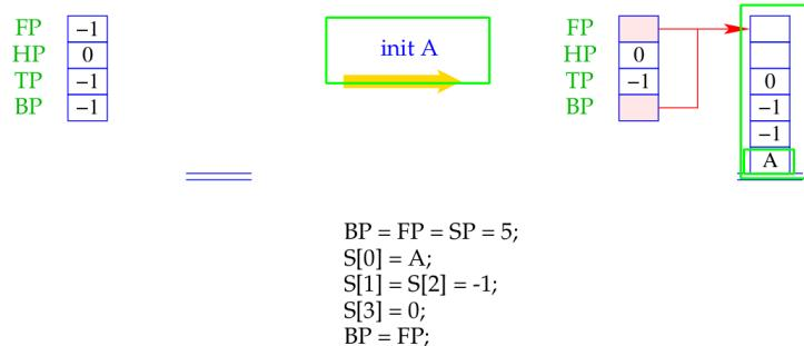
At address "A" for a failing goal we have placed the instruction `no` for printing `no` to the standard output and halt.
