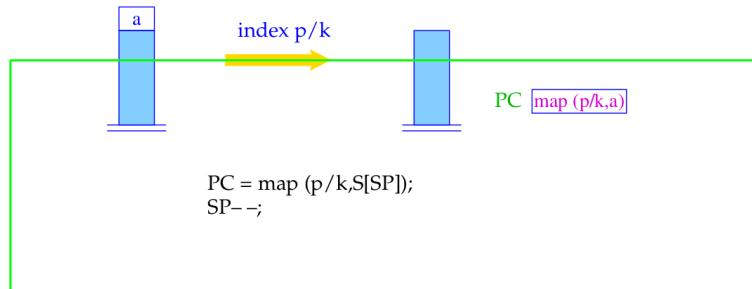
The function `map()` returns, for a given predicate and node content, the start address of the appropriate try chain.
