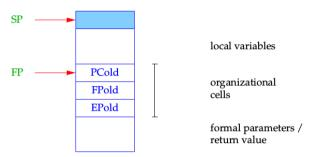
$FP \cong Frame$  Pointer; points to the last organizational cell and is used for addressing the formal parameters and local variables.
