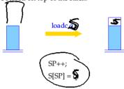
Instruction  $loadc\ q$  needs no operand on top of the stack, pushes the constant q onto the stack.
