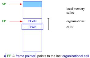
used to recover the previously active stack frame
